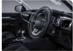
Steering Adjustment With the tilt telescopic feature to adjust the position to make it more comfortable for anyone. (All Type Double Cabin; Single Cabin DSL 4x4 Type)
